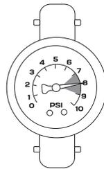
Pump attachments should be configured as shown. The pressure release valve will engage once 9 PSI is achieved.
